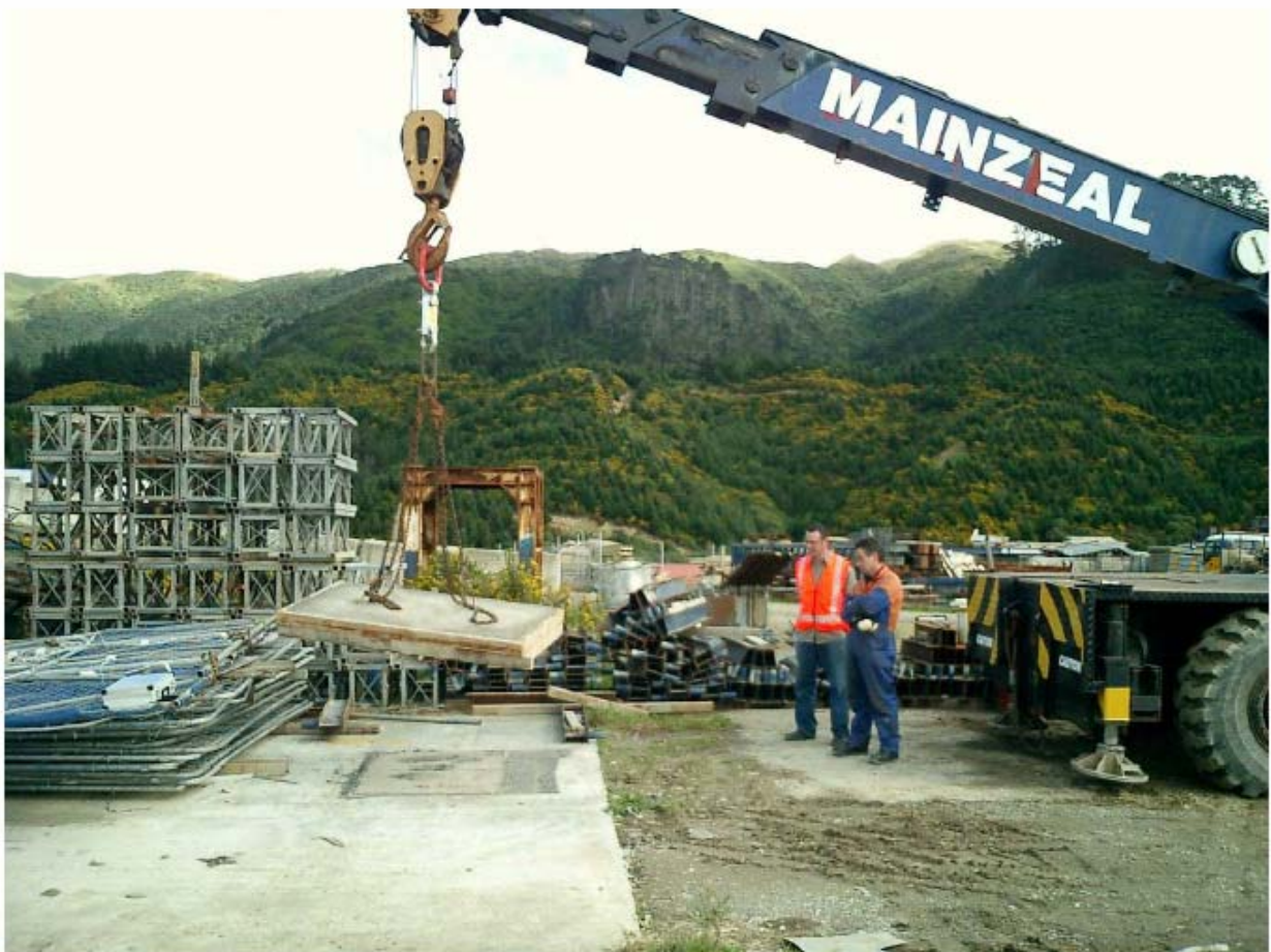
Concrete slab pulled to fail,
